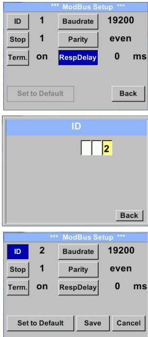
For changes, e.g. the sensor ID, first select by pressing key „ $\Delta$ “ the field “ID” and then key “OK”.
