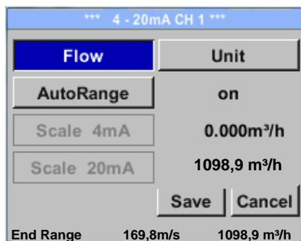
The 4-20 mA Analogue output of the Sensor VA 500 can be individually adjusted.
