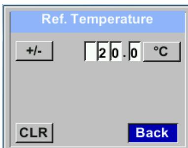
By pressing „ $\Delta$ “ the position value is incremented by 1. Complete with “OK” and activate next number position.
