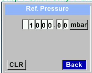
In order to change, e.g. the unit, first select by pressing key „ $\Delta$ “ the field “Units” and then key “OK”.
