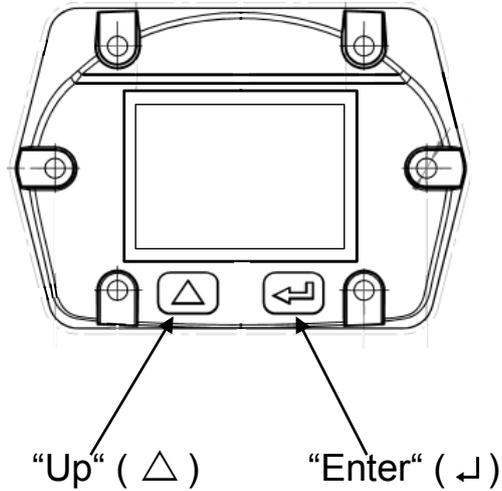
The operation of the VA 500 is done by the two capacitive key buttons Up ( $\triangle$ ) und Enter ( $\leftarrow$ )
