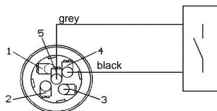
**Remark:** If the sensor is placed at the end of the Modbus system a termination is required. The sensors have an internal switchable termination, therefore the 6 fastening screws from the lid are to be released and set the internal DIP Switch to "On". It must be ensured that the connection plugs are still plugged and the gasket is installed correctly, see also chapter 4.5. Alternatively, a 120R resistor can be installed in the plug between pin 2 and pin 4.
