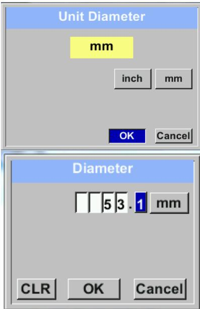
In order to change, e.g. the unit, first select by pressing key „ $\Delta$ “ the field „Units“ and then key „OK“.
