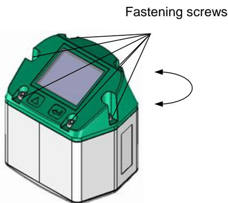
The Position of the Display head is twistable by 180 e.g. in case of reverse flow direction.
