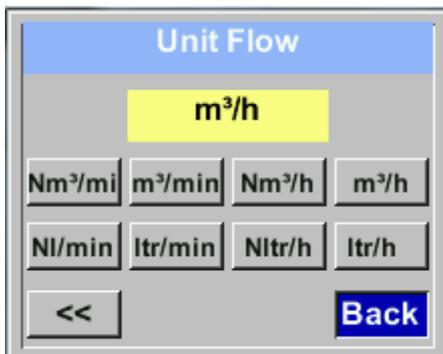
To the selected measurement value a corresponding / appropriate unit needs to be defined. Select „Unit“ with „ $\Delta$ “ and open menu with „OK“. Select required unit with „ $\Delta$ “ and take over by pressing „OK“.
