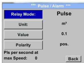
The galvanically isolated output can be defined as pulse- or alarm output. Selection of field „**Relay Mode**“ with key „**Δ**“ and change modus by pressing key „**OK**“.
