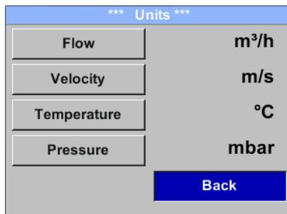
To make changes to the unit for the respective measurement value, first select by pressing „ $\Delta$ “ the field of the „measurement value“ and activate „it with „OK”.
