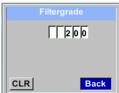
Under point “Filtertime” together with the appropriate “Filter Grade” an attenuation can be defined.
