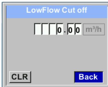
With the low-flow cut off activated, the flow below the defined "LowFlow Cut off" value will be displayed as 0 m<sup>3</sup>/h and not added to the consumption counter.
